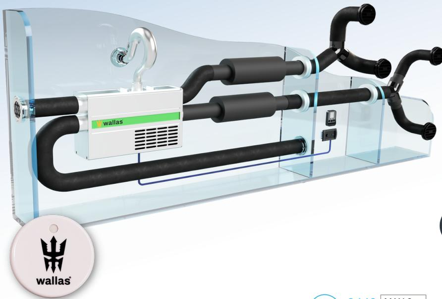
Two inlets take fresh air from outside and recirculate heated air in the cabin. This improves efficiency and ensures oxygen rich air in the cabin.
